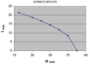
M ax. allo wable ambient Temp. at specific current (rms) B 25667C4197A 375
